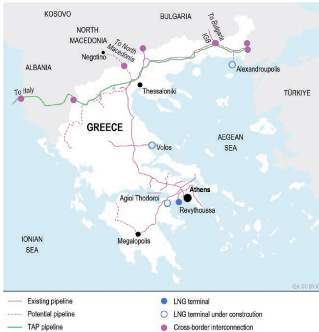
Figure 11: Natural gas infrastructure, source: HAEE
